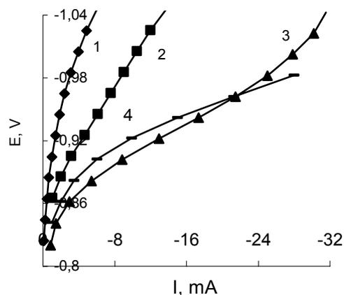
Fig.1. The kinetics of the cathodic process on electrode No. 1 and in the  $\text{LaNi}_{4.5}\text{Mn}_{0.5}$  alloy:
