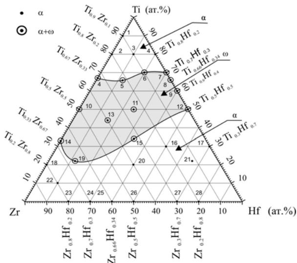
Fig. 2. Concentration triangle of Ti-Zr-Hf system.
