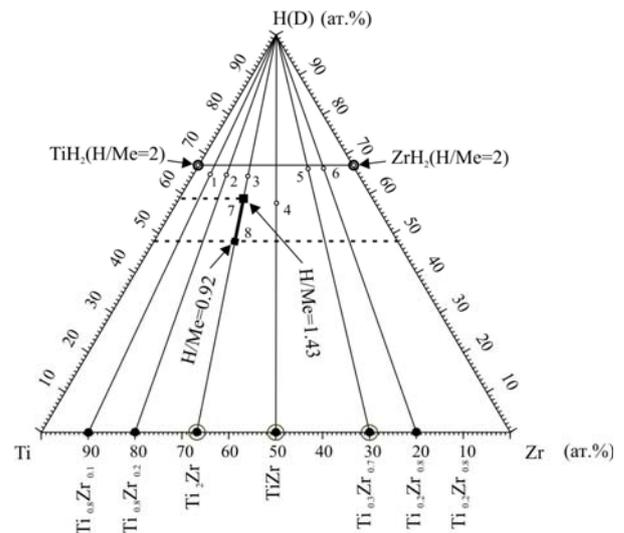
Fig. 1. Concentration triangle of Ti-Zr-H system.
