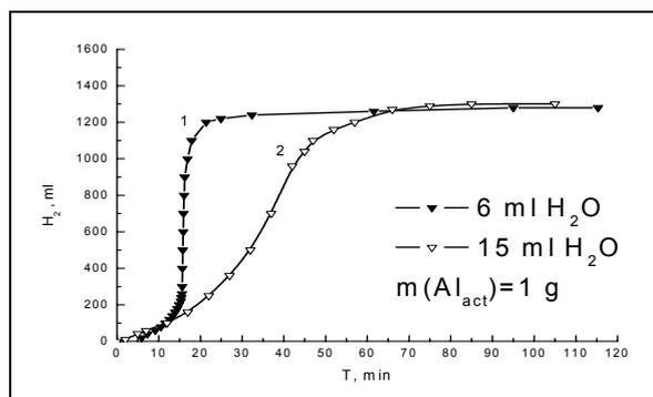
Fig. 2. Dependence of speed of hydrogen allocation on water quantity.
