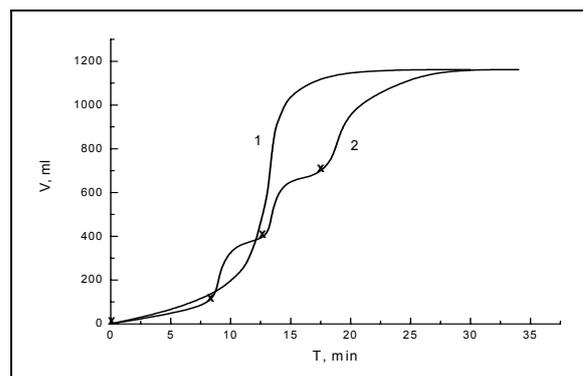
Fig. 4. Addition of water in a reactor at unitary submission (1) and by portion (2).
