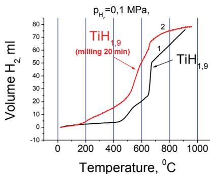
Fig.1. Isobars of the thermal desorption of hydrogen from TiH<sub>1,9</sub> before and after of the dispersion (constant pressure in the reactor - 0,1 MPa).
