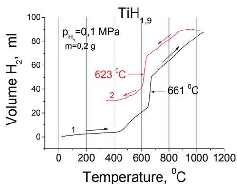
Fig.4. Isobars of the desorption- absorption of hydrogen from initial hydride of  $TiH_{1,9}$  with pressure 0,1 MPa .
