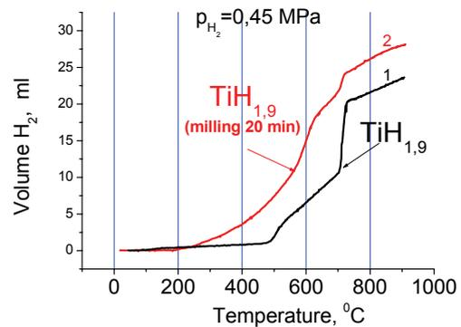
Fig.2. Isobars of the thermal desorption of hydrogen from TiH<sub>1,9</sub> before and after of the dispersion (constant pressure in the reactor - 0,45 MPa).
