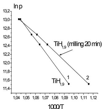
Fig.3. Dependence of the equilibrium pressure hydrogen from reverse temperature for initial hydride of  $TiH_{1,9}$ (1) and subjected to mechanical dispersion hydride of titanium (2).
