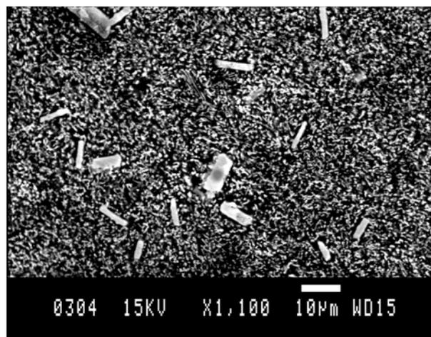
Fig. 2. SEM image (SE mode) of the binary eutectic alloy Mg-Ni, modified by ECAP at 300°C (4 passes, 15 mm/min).
