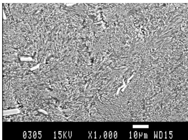
Fig. 1. SEM image (SE mode) of the binary eutectic alloy Mg-Ni, modified by ECAP at 250°C (1 pass, 10 mm/min).
