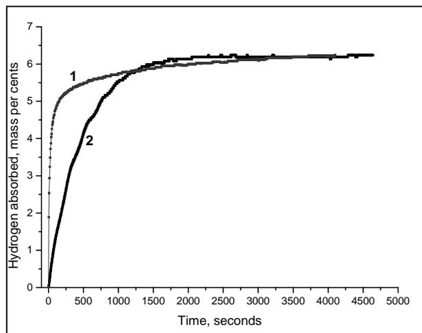
Fig. 3. Hydrogen absorption curves at 350°C by the binary eutectic alloy Mg-Ni: modified by ECAP (1) at 250°C (1 pass, 10 mm/min) and the initial (2).
