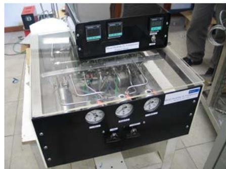
Fig. 4. General view of the MH compressor.
