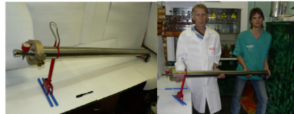
Fig. 4. Compressor of high-pure hydrogen “Svetzag – 2000”.
