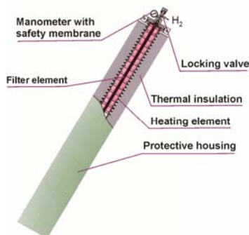
Fig. 3. Schematic view of the laboratory metal hydride storage/compressor of high-pure hydrogen “Svetzag – 2000”.
