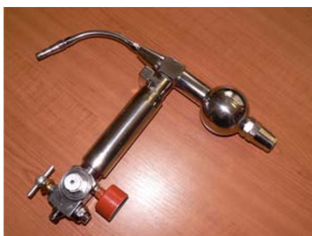
Fig. 5. The oxydric torch with metal-hydride accumulator of hydrogen, cylinder of high pressure for oxygen and piezoelectric firing of flame.
