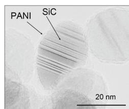
Fig.1. TEM image of nc-SiC functionalized at the surface by nanometric layer of PANI-CSA.
