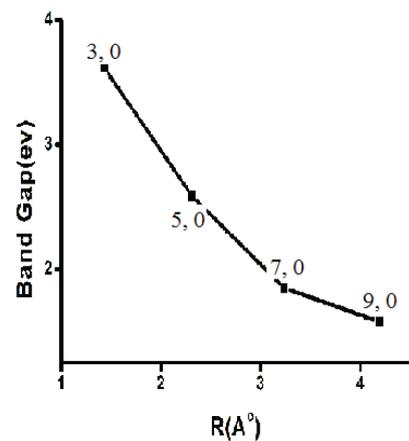
**Fig.4** Variation of the band gaps after hydrogenation in terms of the tube's radii.
