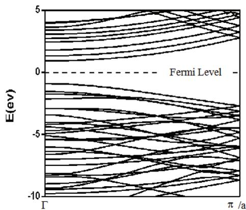
**Fig.3** Band structure of the (7, 0) SWCNTs after hydrogenation.
