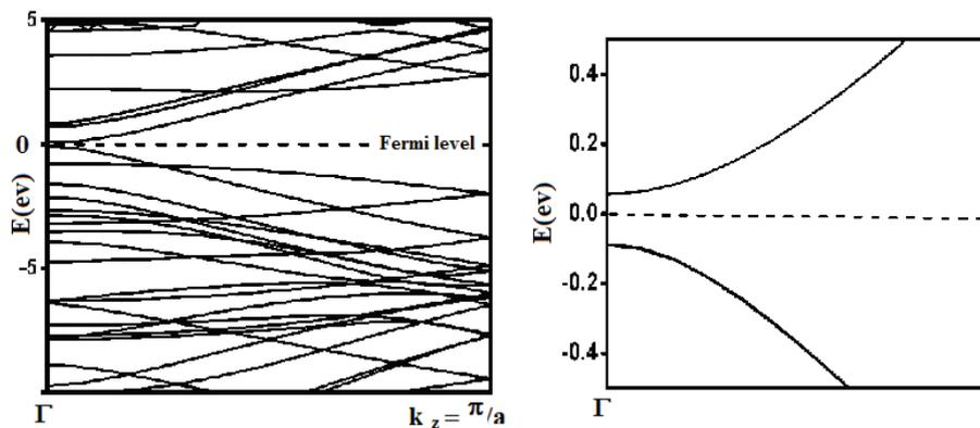
**Fig.2** Left- Band structure of (7, 0) SWCNT; Right- Magnification of the Fermi level area in the left graph.
