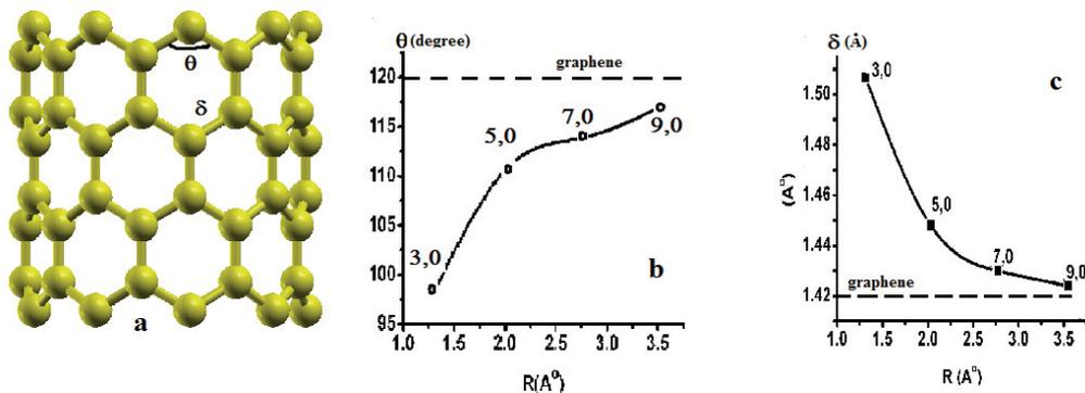
Fig.1 (a)- a zigzag SWCNT with specifying of  $\theta$  and  $\delta$  parameters; (b) & (c) - variation of the  $\theta$  and  $\delta$  parameters in terms of the tube's radii.
