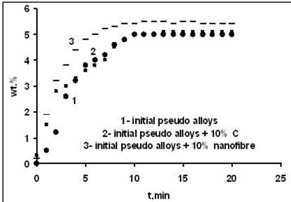
Fig. 2. Curves of hydrogen sorption by "pseudoalloy" (1) and "pseudoalloys" added with graphite (2) and nanofibers (3).
