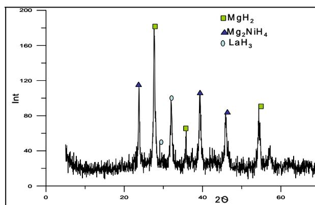
Fig. 1. X-ray diffraction pattern (CuK<sub>α</sub>) of the hydrogenated composite of the "pseudoalloy" with 10 mass% of graphite.
