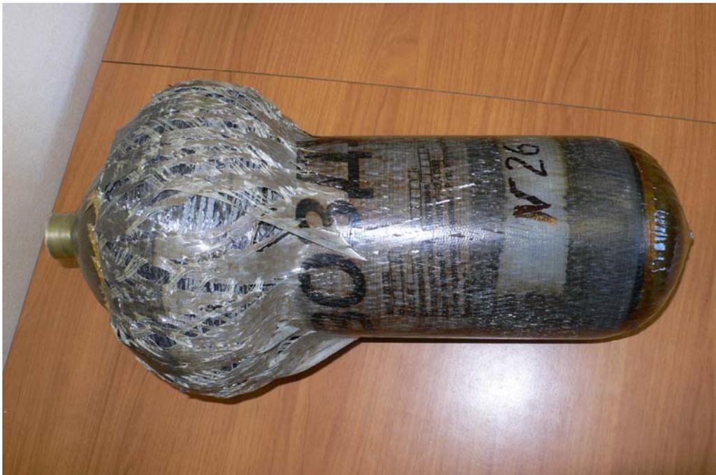
Fig. 2. The nonshattering character of the composite tanks and bottles breakdown.
